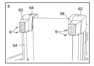
Make sure that all parts are properly tightened before you use the treadmill. Note: Extra hardware may be included. Keep the included allen wrenches in a secure place. The large allen wrench is used to adjust the walking belt (see page 23). To protect the floor or carpet, place a mat under the treadmill.
